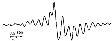
Fig. 3. EPR spectrum of a mixture of cation radical I^{\cdot+} and the chloranil anion radical in the I-chloranil system in acetonitrile.
